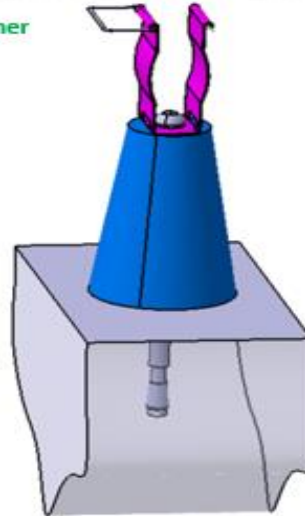
Assembly with 1/2" SS Clamp
